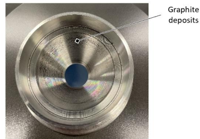
Figure 10. Graphite deposits after contact event testing
