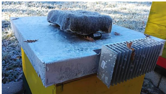
Figure 6. In-situ testing of the prototype energy harvesting system
