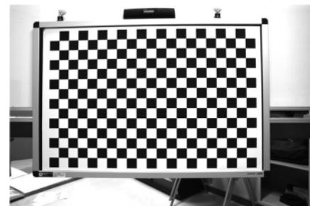
Figure 3. Grid pattern for conventional camera calibration.
