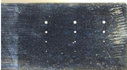
Figure 6. Subsequent prototype hole pattern under stereo microscope
