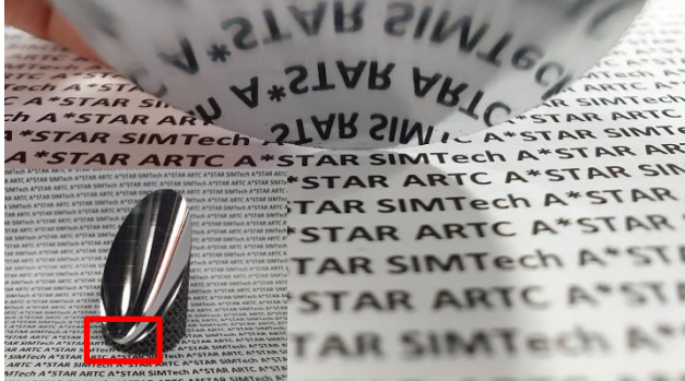
Figure 9. The ultraprecision lightweight freeform mirror
