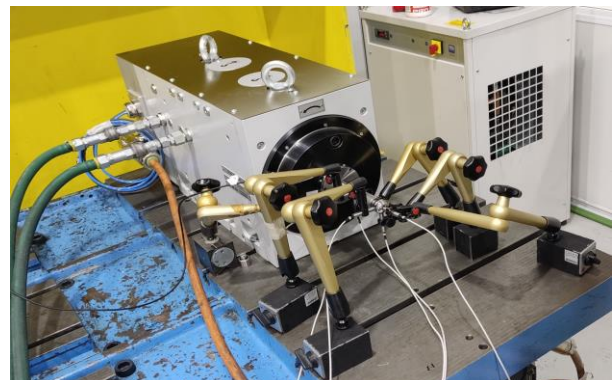
Figure 1. Test bench for the measurement of rotational error of spindles.
