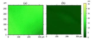
**Figure 1.** Noise map of 50× magnification objective lens configuration obtained using the subtraction method for (a) CM and (b) CSI mode.
