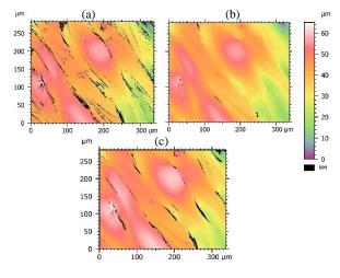
**Figure 3.** Surface topography map of an AM surface ( $Sq \approx 9 \ \mu m$ ) obtained using (a) CM, (b) FV and (c) CSI modes.
