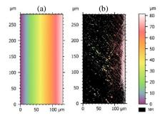
**Figure 2.** Surface topography map of a 30° tilted optically smooth surface obtained using (a) CM and (b) CSI modes.
