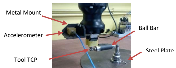
Figure 1 COBOT End Effector Setup
