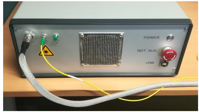
Figure 3. 19"-housing for OCT components.
