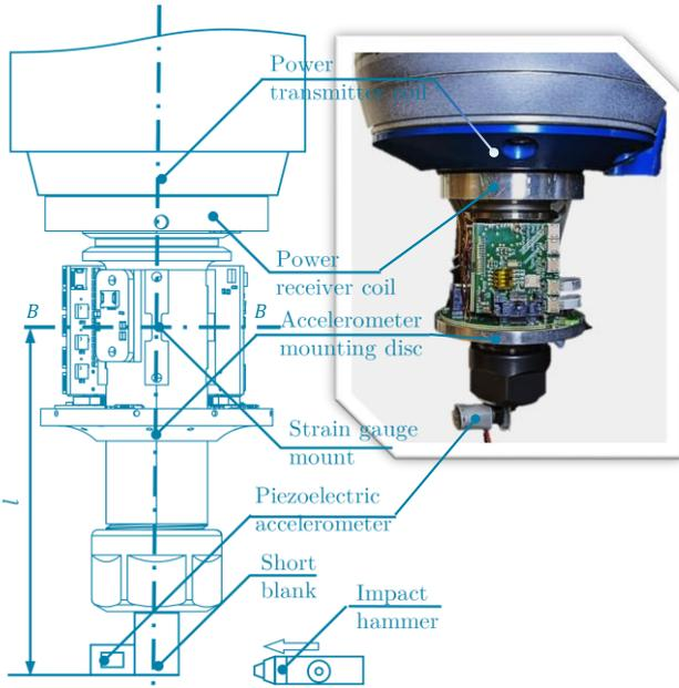
**Figure 4.** Schematic of the instrumented tool holder clamped in the machine spindle. Left: the strain gauges along  $BB$  axis measure the applied moment from instrumented hammer. A similar perpendicular  $AA$  axis is also measured simultaneously for cross-talk estimation. Right inset: Photograph of the setup.
