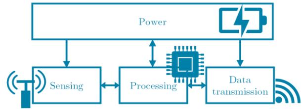
Figure 2. Function blocks of the sensing tool holder
