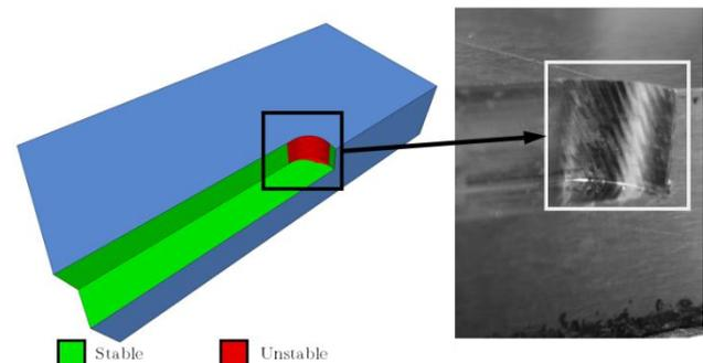
**Figure 9.** Left: Visualization of location of chatter, right: chatter marks seen on the workpiece
