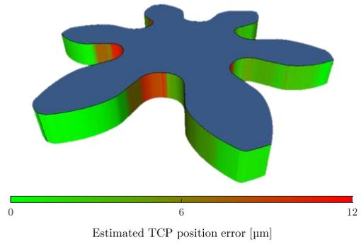
**Figure 8.** Estimated TCP deviation plotted on gear profile.
