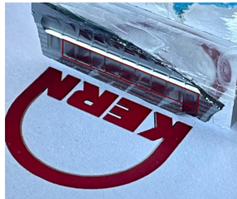
Figure 8: The milled sample. The ball end milled region is highlighted with a red square. Note the much clearer reflection in this area compared to the rest of the sample specimen.
