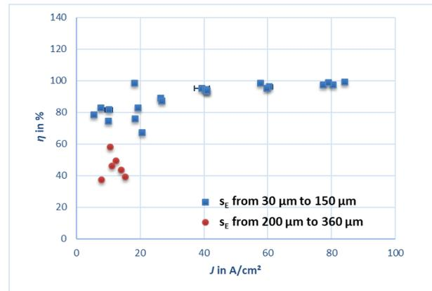
**Figure 6.** Current efficiency as function of current density
