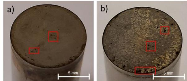
**Figure 2.** Surfaces of samples machined with different current densities; a) 10.0 A/cm<sup>2</sup>; b) 40.4 A/cm<sup>2</sup>
