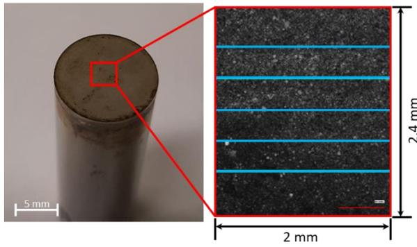
**Figure 3.** Representation of the surface quality measurement
