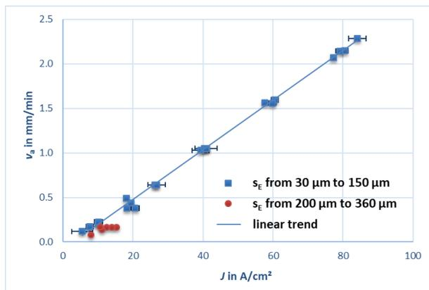
**Figure 5.** Removal rate as function of the current density of the material NdFeB for different gap size
