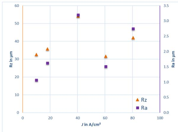
**Figure 4.** Roughness  $Rz$  and  $Ra$  over current density
