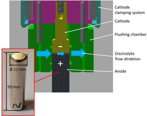
**Figure 1.** CAD model of the ECM device used for analysis of the removal characteristic with an unmachined sample
