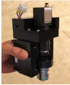
**Figure 1.** Optical profilometer sensor. It was designed to minimize dimensions and weight.
