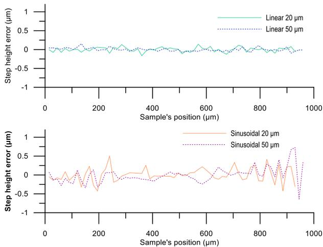
**Figure 2.** Step height error obtained from measuring a step placed in different positions along the scanning range (1 mm), using a linear movement profile (top) and a sinusoidal profile (bottom).
