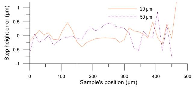
**Figure 3.** Step height error obtained from measuring a step placed in different positions along the scanning range (500  $\mu\text{m}$ ), moving with a sinusoidal profile.
