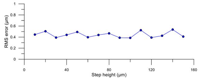
**Figure 4.** RMS of the step height error through different positions of the axial scan with different values of step height when using a sinusoidal movement profile.
