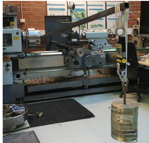
Figure 3. Maximum static throughput torque was measured by using a beam and an accurately known mass. The figure presents the unloaded situation where the mass is hanging from an overhead crane.
