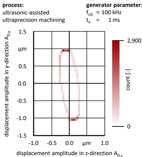
Figure 2. Displacement amplitude  $A_D$  in TCP-coordinates
