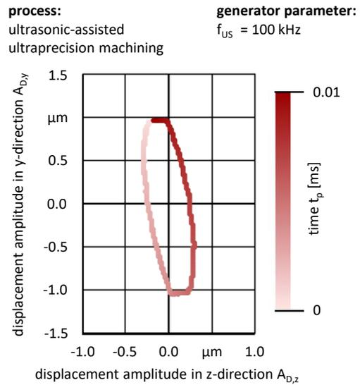
Figure 3. Time depended TCP-coordinates of the displacement amplitude  $A_{D,y}$  and  $A_{D,z}$
