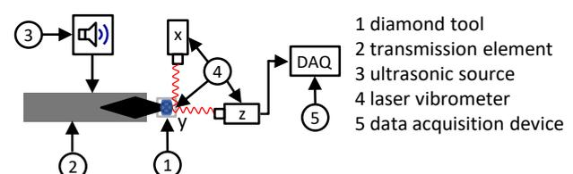
Figure 1. Schematic overview of the sensorised measurement setup
