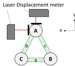
Figure 3. Measurement method using a laser displacement meter
