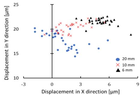
Figure 5. Plot of the displacement of inchworm per one cycle.
