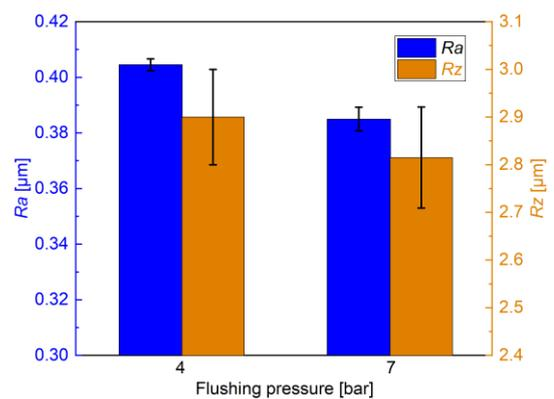
**Figure 4.** Effects of the flushing pressure on the surface roughness
