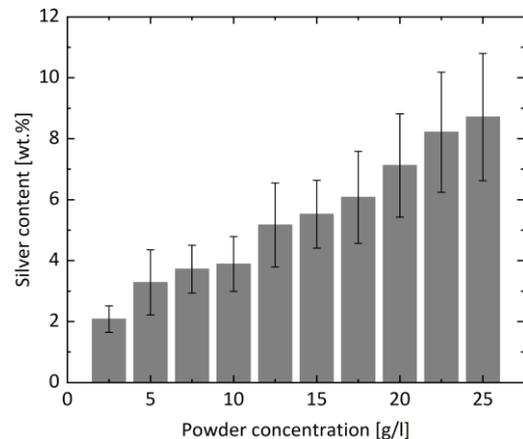
**Figure 1.** Influence of the powder concentration in the dielectric fluid on the deposited silver content. Machining conditions: lateral flushing, hollow tool electrode with outer diameter of 0.6 mm and inner diameter of 0.17 mm, 10  $\mu$ J discharge energy, positive tool electrode [4].
