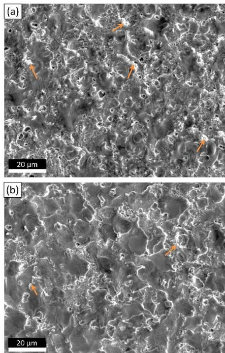
**Figure 9.** SEM images of workpiece surfaces modified using 7 bar pressure: (a) spectrum 1 and (b) spectrum 8. Orange arrows point on the regions (identical areas to Fig. 8) with spattered silver
