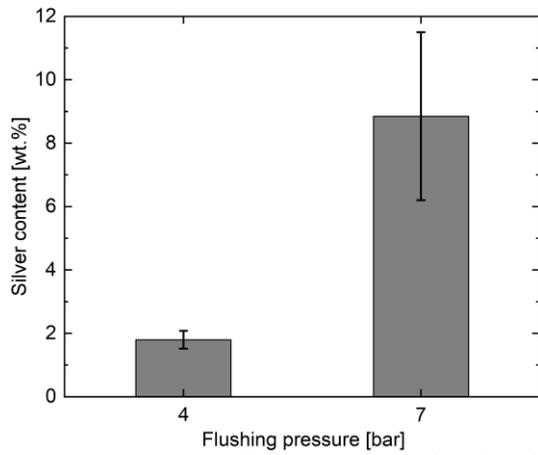
**Figure 5.** Deposited silver content on workpiece surfaces for different flushing pressures
