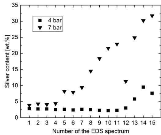
**Figure 6.** Distribution of deposited silver over the modified surfaces
