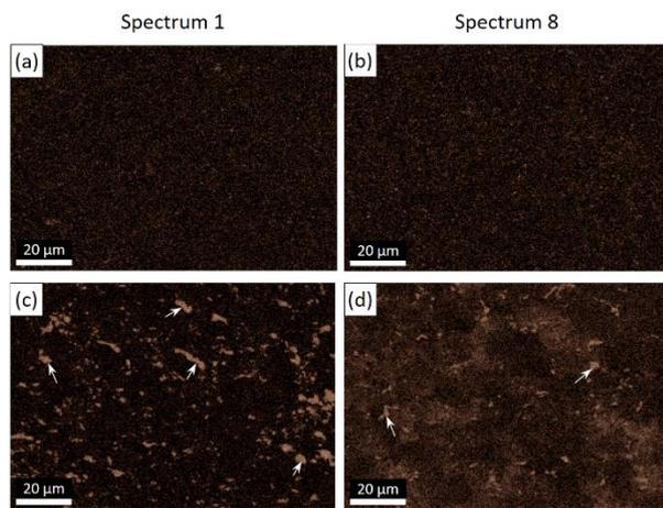
**Figure 8.** Silver mapping of workpiece surfaces modified using 4 bar (a-b) and 7 bar (c-d) of the dielectric pressure. Arrows point on the areas with silver clusters
