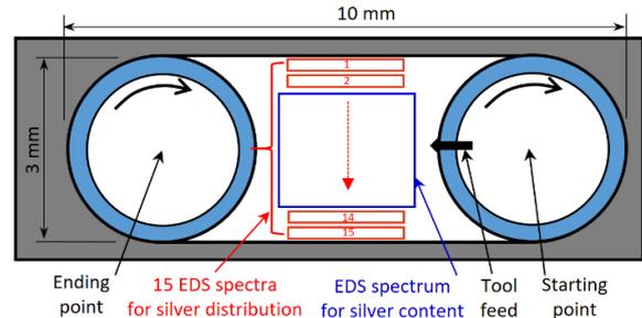
**Figure 3.** Schematic showing the geometry of the machined areas and locations for EDS spectra analyses of the silver content and silver distribution
