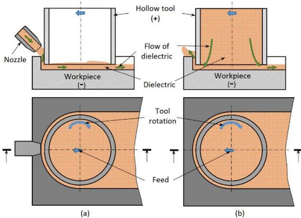
**Figure 2.** Schematic showing the difference between (a) lateral flushing and (b) internal flushing
