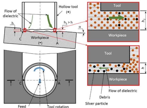
**Figure 7.** Change of the machining gap caused by non-parallelism of tool tip surface and workpiece surface, effects on the dielectric flow and the amount of silver powder as well as debris particles in the gap. Thicker arrows mean higher flow rate. Points C and A are positions of the analysed spectra 1 and 15, respectively
