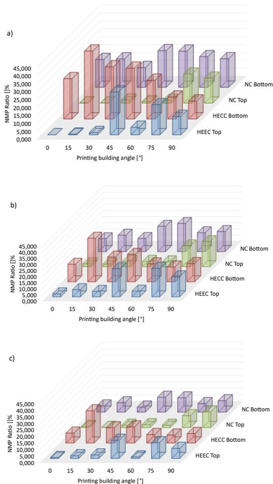
**Figure 5.** Non-measured points ratio (NMP) assessment for different optical measurement methods: (a) CSI, (b) CSM, (c) CF
