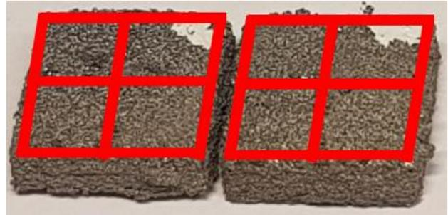
**Figure 3** The demonstration of the location of supporting structures as highlighted in the red zones.
