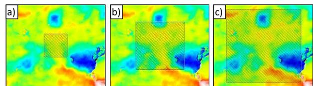
**Figure 6.** different cut-off size of over the surface area (338 µm x 284 µm): (a) 80 µm, (b) 165 µm, (c) 250 µm, contributing to filtering and separation of roughness and waviness.
