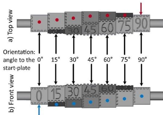
**Figure 1.** The design of the artefact with a) top view and b) front view. The red dots and arrows in a) demonstrate the up-facing surfaces while the blue ones in b) indicate the downfacing surfaces.
