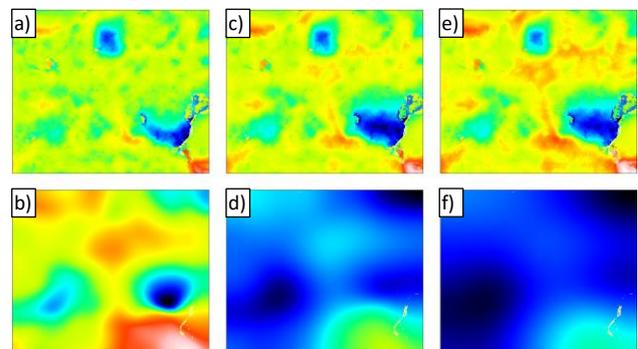
**Figure 7.** Roughness and waviness after using RGRF with three different cut-offs: (a, b) 80 µm, (c, d) 165 µm (e, f) 250 µm.
