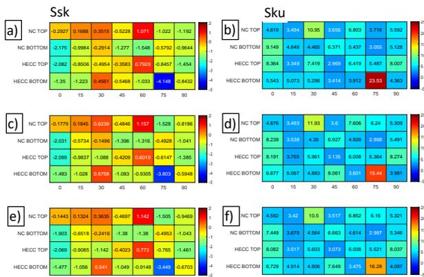
**Figure 8.** Heatmap representation of skewness (*Ssk*) and kurtosis (*Sku*) for three optical measurement methods: (a, b) CSI, (c, d) CSM, (e, f) CF. The X-axis represent the build angle in deg, Y-axis represents surfaces after different printing strategies (non-contouring and contouring).
