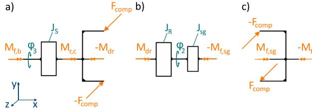
Figure 2. Mechanical model of a) stator. b) rotor. c) MSD.
