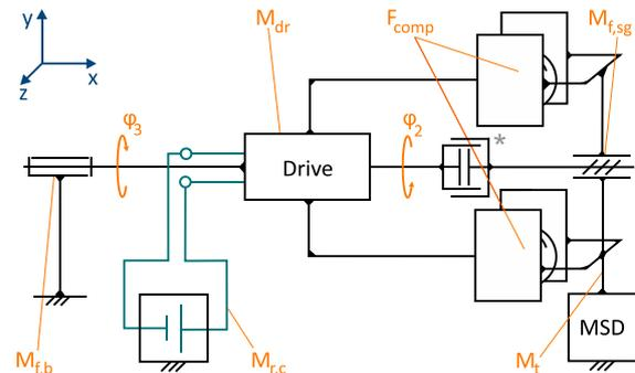
Figure 1. Simplified working principle. (\*shiftable form-fit coupling)
