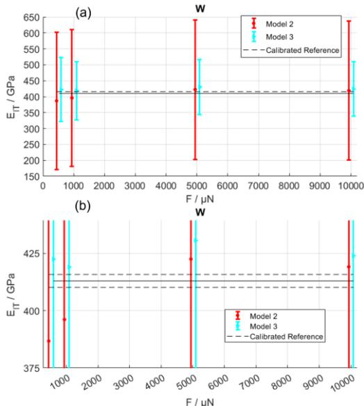
**Figure 6.** Comparison of characterisation of tungsten (W) indentation modulus  $E_{IT}$ ; only models #2 and #3 (shown in Table 1) are reported, for the others introduce a significant systematic difference or are too dispersed. (b) is a magnified view.
