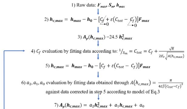
**Figure 3.** Calibration iterative procedure workflow.
