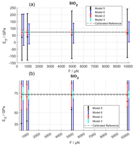
**Figure 5.** Comparison of characterisation of fused silica (SiO<sub>2</sub>) indentation modulus  $E_{IT}$ ; models #1 and #4 (shown in Table 1) are unreported for they introduce a significant systematic difference. (b) is a magnified view.
