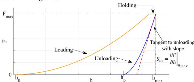
Figure 1. Example of IC showing relevant parameters.
