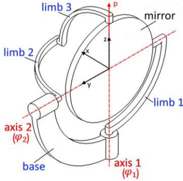
Figure 2. Kinematic structure of a spherical 5R parallel mechanism.
