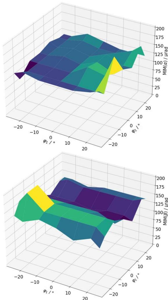
**Figure 7.** Achievable minimum incremental motion for the tip/tilt angles  $\alpha$  and  $\beta$  for different input angles  $\varphi_1$  and  $\varphi_2$ .
