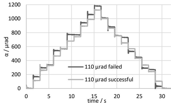
Figure 6. Measurement results for successful and unsuccessful minimum incremental motion tests. Here, steps with 110  $\mu\text{rad}$  step sizes are made and the mechanism's response is measured.
