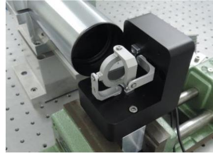
Figure 5. Measurement setup for the experimental investigation of the high-precision tip/tilt mirror.
