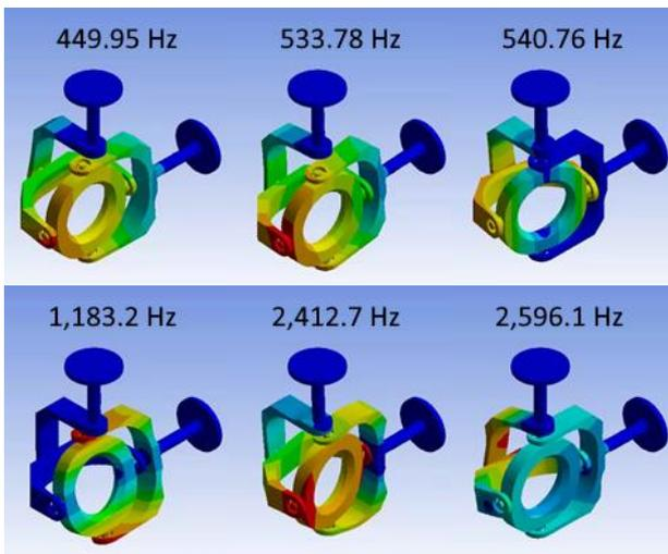
Figure 4. Eigenfrequencies and their corresponding Eigenmodes of the high-precision tip/tilt mirror.
