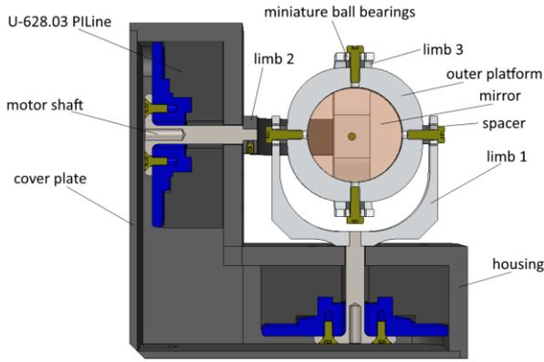
Figure 3. Components and assembly of the high-precision tip/tilt mirror.
