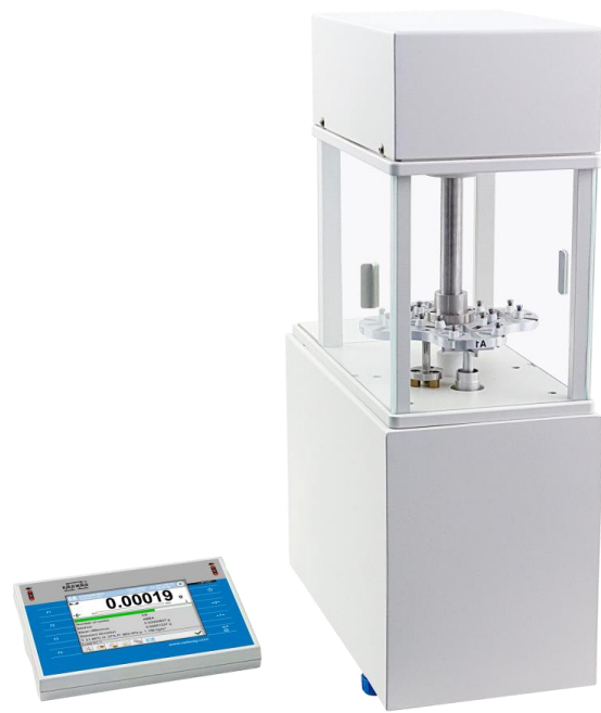
Figure 4. View of the novel AK-4 mass comparator with readability of 10 ng
