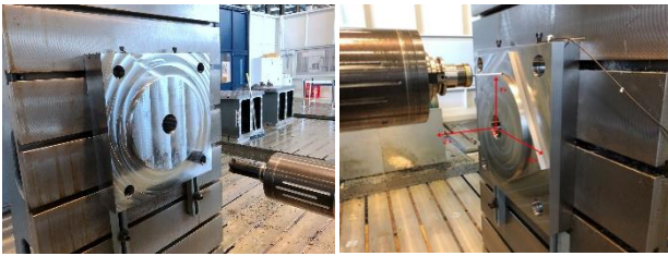
Figure 3. Workpiece manufacturing and on-machine tool measurement
