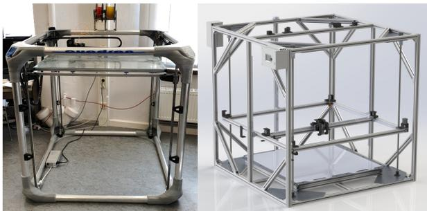
Figure 1. a) existing system, b) rendering of the new designed fff-printer
