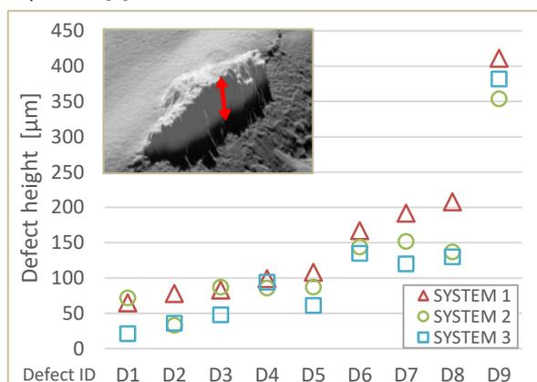
Figure 1. Example of surface defect height measurements
