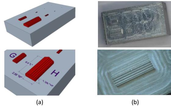
**Figure 3.** Final design (a) and prototype (b) of the specimen
