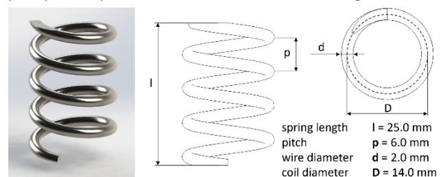
Figure 1. CAD-rendering and design parameters of the samples
