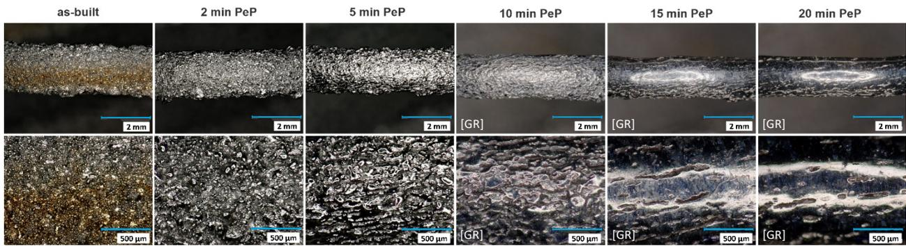
**Figure 2.** Optical micrographs of the lateral spring surface (centre coil) after different PeP times; [GR] recorded with active gloss reduction
