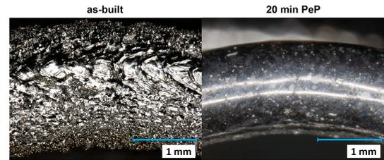
**Figure 3.** Optical micrographs of the upskin surface before and after PeP
