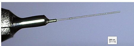
Figure 3. The dressed electrode by WEDG unit. Image acquired through a digital microscope (Dino-Lite® Edge AM4115ZT)
