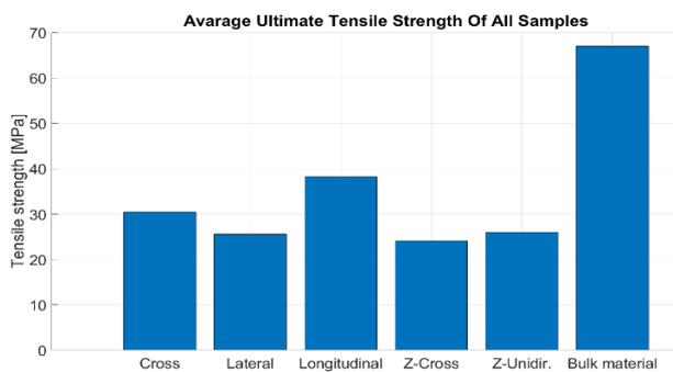
**Figure 4.** Mean UTS for each of the five sample types tested, as well as UTS of stock shape bulk material taken from the datasheet [3].
