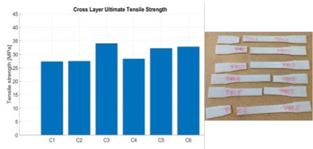
**Figure 5a.** Cross layered tensile test specimen UTS results (left) and broken samples (right).
