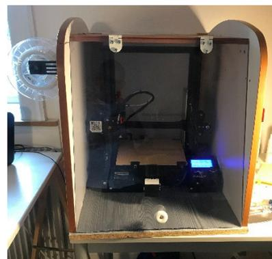
Figure 1. Printer with enclosure.
