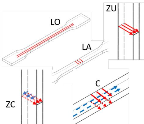
**Figure 2.** The figure shows how print direction is varied in the samples. **LO:** longitudinal, **LA:** lateral, **C:** cross layered, **ZU:** unidirectional z-print and **ZC:** cross directional z-print.
