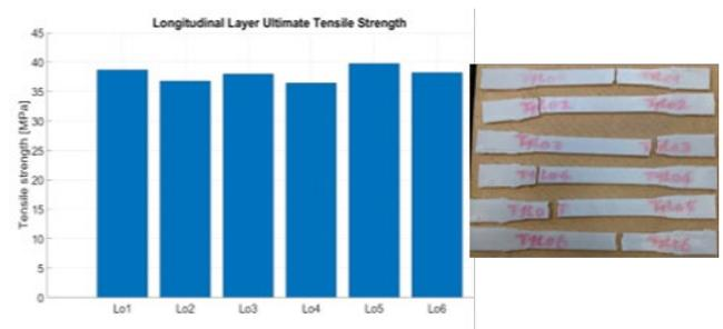
**Figure 5c.** Longitudinally printed tensile test specimen UTS results (left) and broken samples (right).
