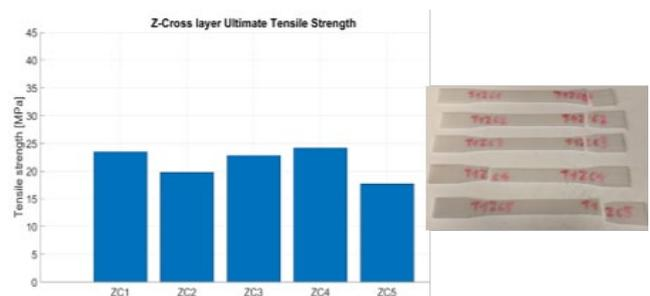
**Figure 5d.** Cross-layered, vertically printed, tensile test specimen UTS results (left) and broken samples (right).
