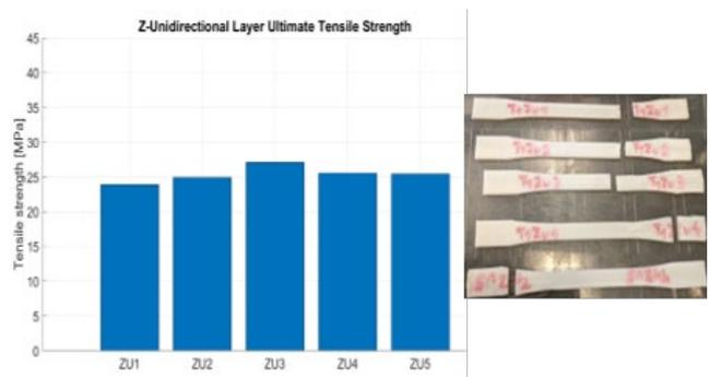
**Figure 5e.** Unidirectionally-layered, vertically printed, tensile test specimen UTS results (left) and broken samples (right).
