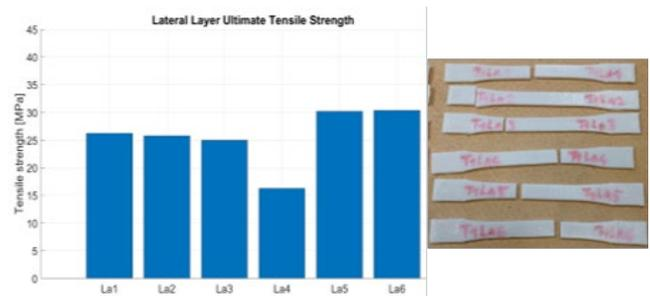
**Figure 5b.** Laterally printed tensile test specimen UTS results (left) and broken samples (right).
