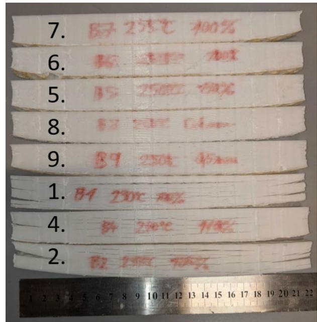
**Figure 3.** The figure shows beam samples printed at different temperatures and flowrates.
