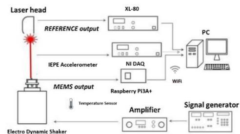
Figure 2 Calibration Test Rig
