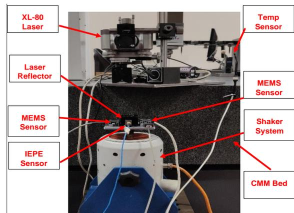
Figure 1 Calibration Test Rig
