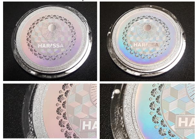
Figure 4. photograph of an aluminium coated replica. Left) made with optimized parameter right) made without injection compression.
