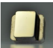
Figure 2. CrN coated mold insert
