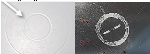
Figure 2. Wear track on the PTFE sample (on the left) and wear track appearance on the aluminium sample (on the right) after a rotary pin-on-disc test
