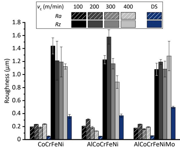
**Figure 1.** Influence of the material and the cutting speed in face turning as well as the effect of diamond smoothing on  $R_a$  and  $R_z$
