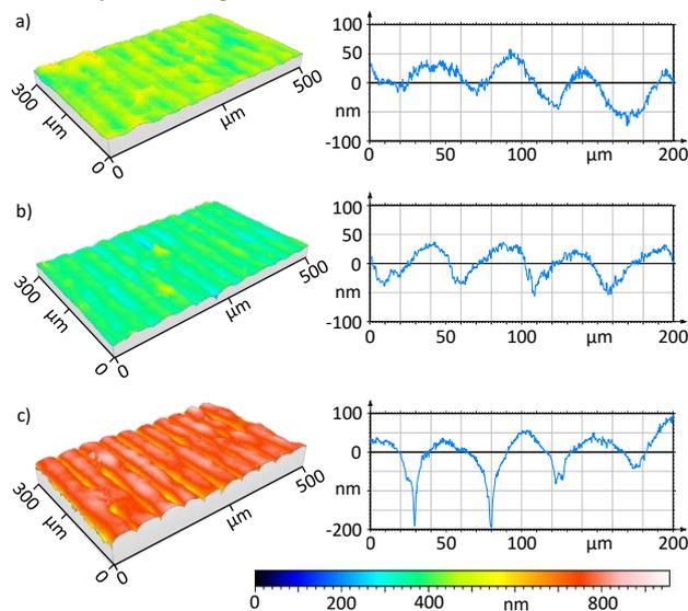
**Figure 3.** Surfaces detected by 3D LSM after diamond smoothing of CoCrFeNi (a), AlCoCrFeNi (b), and AlCoCrFeNiMo (c) (2D profiles are detected in the direction of feed motion)
