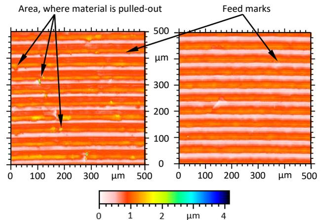
**Figure 2.** Surfaces detected by 3D LSM after machining CoCrFeNi with a cutting speed of 100 m/min (left) and 400 m/min (right)
