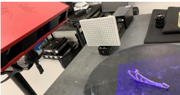
Figure 2. The optical fringe projection measurement system GOM Atos Core 300 while measuring the selected test part
