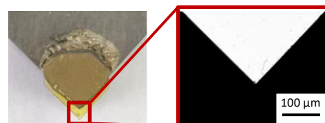
Figure 2. Single crystal diamond tool with the nose angle of 90°
