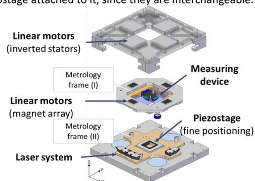
Figure 1. Exploded view of the NanoPla.
