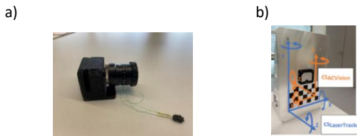
Figure 10. The ACVISION prototype realization; a) Photogrammetry and autocollimation in a single camera device, b) special artefact for the object tracking. Image: TEKNIKER.
