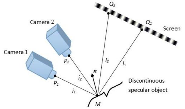
Figure 2. Stereo deflectometry schematic diagram
