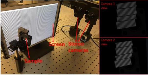
Figure 4. Set up of stereo deflectometry.
