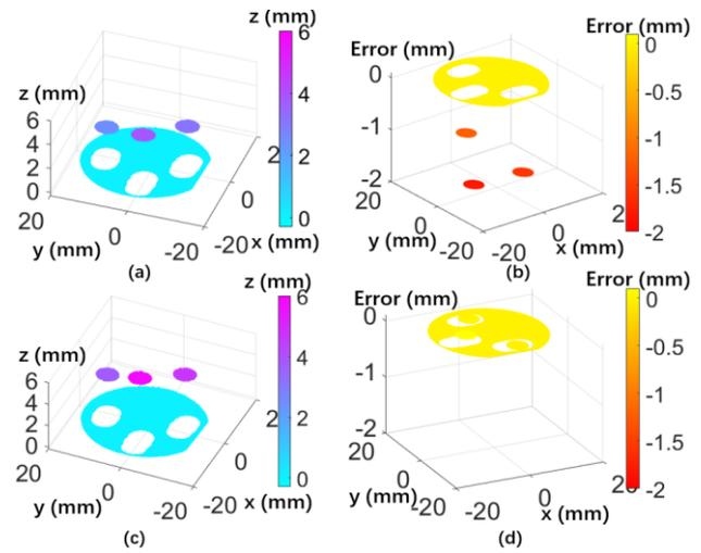
Figure 6. Comparison of measurement data of a specular circle mirror. (a) Original measurement result before compensation; (b) error of original measurement; (c) measurement data after compensation; (d) error of compensated measurement data.
