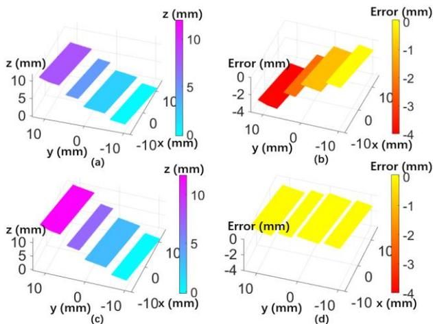
Figure 5. Comparison of measurement data of a specular step gauge. (a) Original measurement result before compensation; (b) error of original measurement; (c) measurement data after compensation; (d) error of compensated measurement data.
