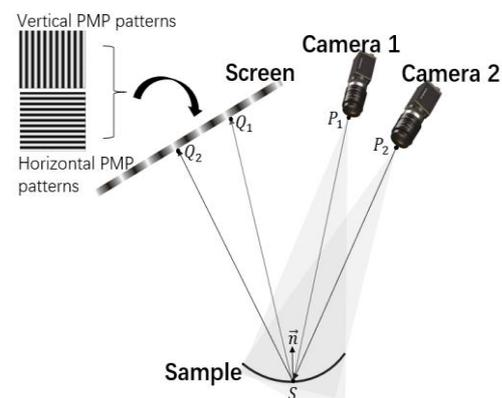
Figure 1. Illustration of measurement principle of stereo deflectometry.
