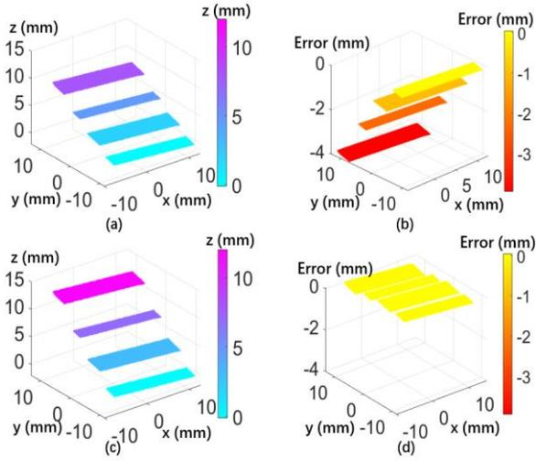
**Figure 2.** Comparison of measurement data. (a) Original measurement result before compensation; (b) error of original measurement; (c) measurement data after compensation; (d) error of compensated measurement data.
