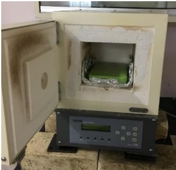
Figure 7. Heat solidification equipment for carbon.
