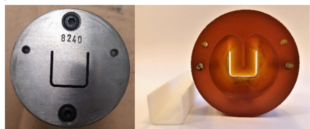
Figure 1. On the left, the flat steel die showing the profile selected for the experiments. On the right, die B with the new conical design and with the extrudate produced.
