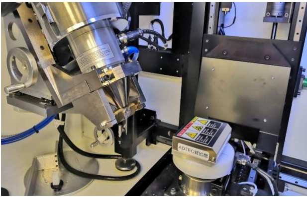
Figure 1. Experimental setup for XCT of torch
