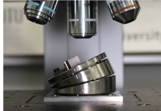
Figure 5. The manufactured precision fixture in a measurement situation with a confocal laser scanning microscope where the surface roughness of a sidewall geometry of a protruding feature is being evaluated.
