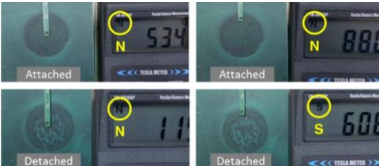
Figure 5. Magnetic views of AlNiCo magnet attached and detached
