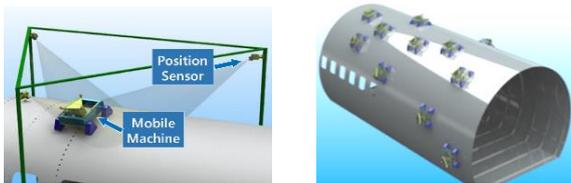
Figure 1. A mobile machine on machining on-site and multi-collaborative machining
