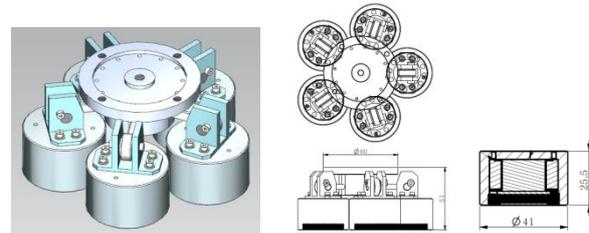
Figure 7. Design of EPM chuck set for curved surface
