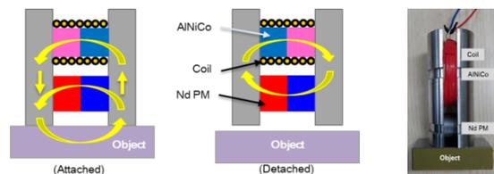
Figure 2. Magnetic circuit with AlNiCo magnet and Nd permanent magnet for attaching and detaching
