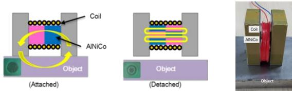
Figure 4. Magnetic circuit with only AlNiCo magnet for attaching and detaching
