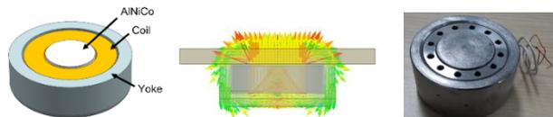
Figure 6. EPM chuck with only AlNiCo magnet for attaching and detaching
