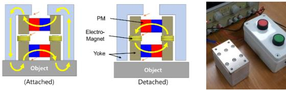
Figure 3. A commercial switchable permanent magnetic chuck
