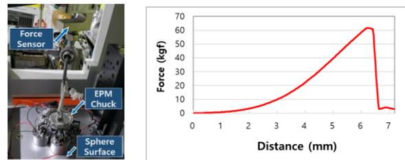
Figure 8. An experiment of the EPM chuck set on sphere surface
