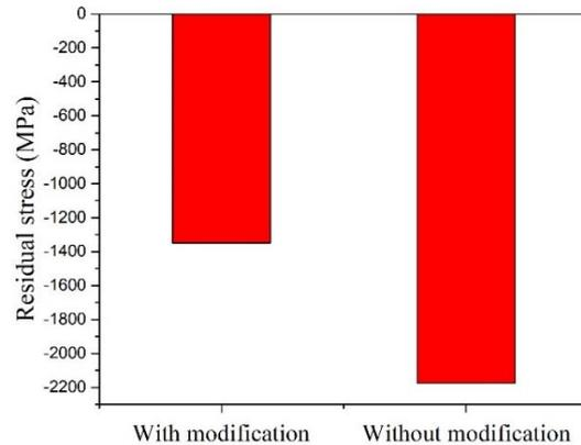
Figure 5. Residual stresses after the grinding experiments.
