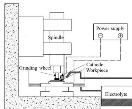
Figure 1. Experimental setup for grinding with electrochemical modification.
