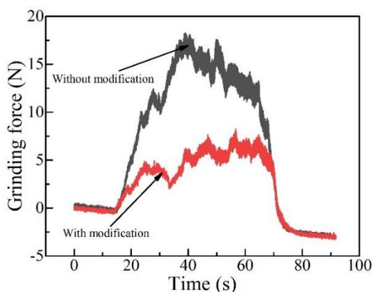
Figure 4. Forces in the grinding experiments.
