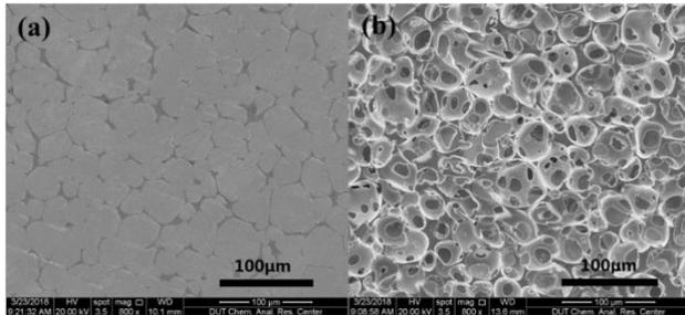
Figure 2. Morphologies of the workpiece before (a) and after (b) modification.
