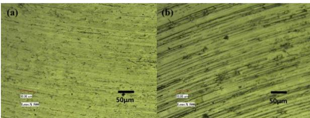
Figure 3. Morphologies of the workpieces after grinding with electrochemical modification (a) and without modification (b).
