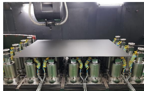
Figure 1. Developed 5-axis machining center and universal jig and fixture
