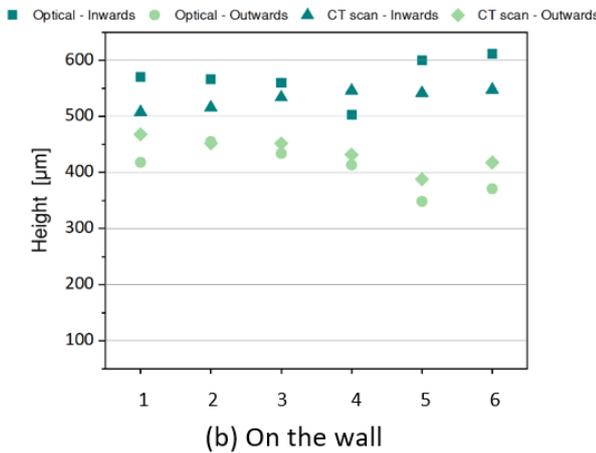
**Figure 3:** Height and depth of the micro pyramids measured with the optical microscope and CT scan for both inwards and outwards pyramids on the bottom and on the wall.
