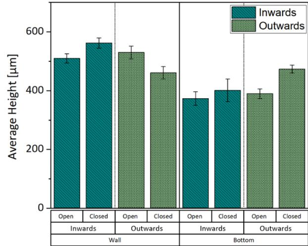
**Figure 4:** Average height of micro pyramids on the wall and bottom in the open and closed mould respectively. Error bars indicate the standard deviation of the height calculate from six pyramids.
