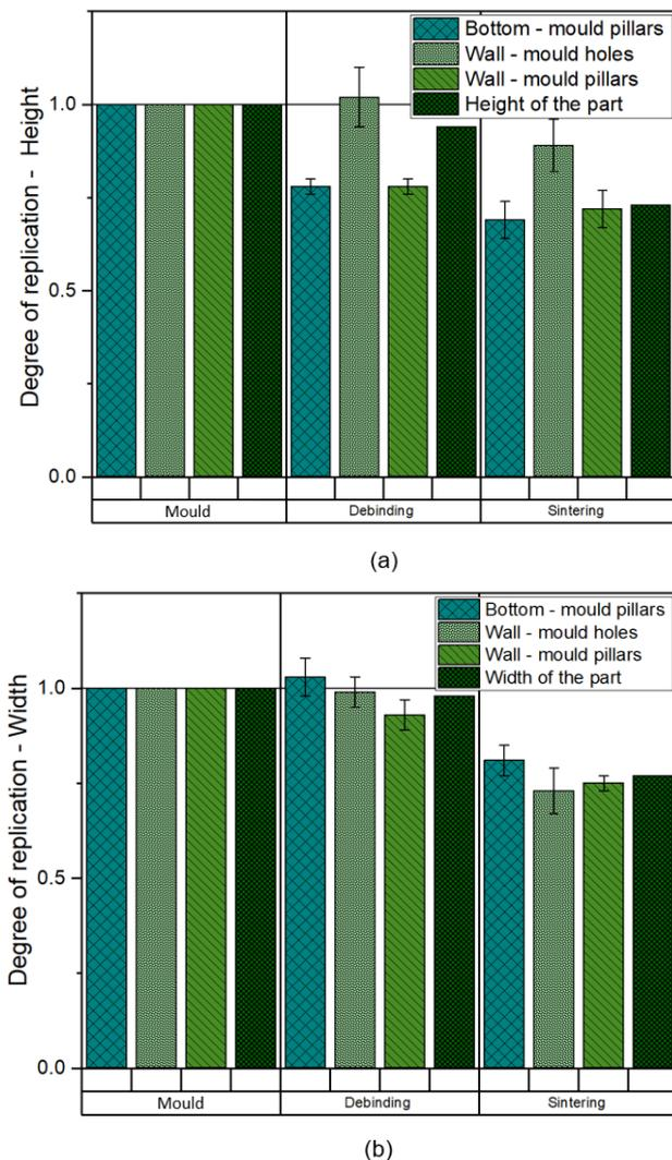
**Figure 5:** Replication rate in the process chain of: height of the overall part and height of microstructure in (a), and overall width of the part and width of the microstructure in (b).
