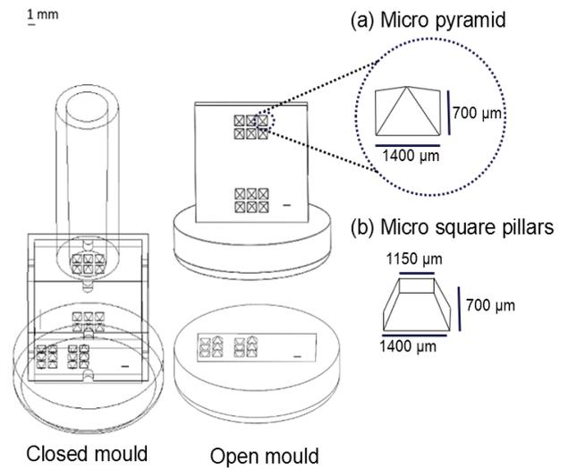
**Figure 2:** Closed mould with pyramid structure on the left, two open moulds for optical measurements on the right. Another version with micro square pillars was also created to study the degree of replication in the process chain.
