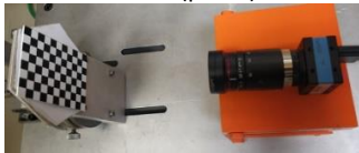
Figure 3. Camera calibration setup using artefact
