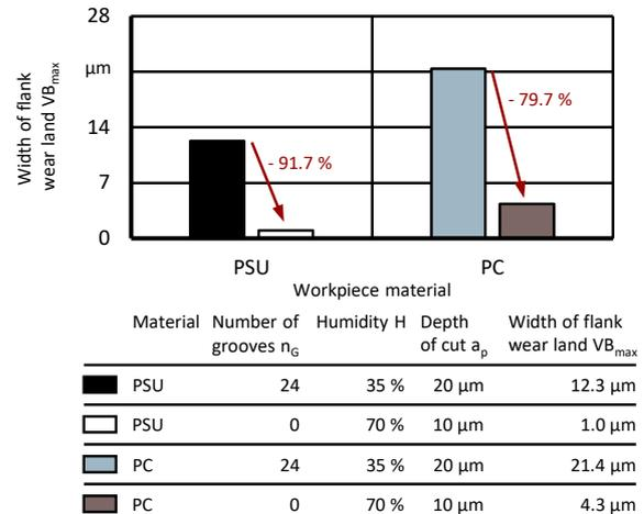
**Figure 3.** Highest and lowest tool wear in PSU and PC
