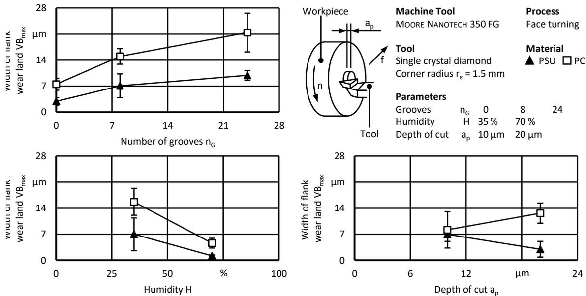
**Figure 2.** Diamond tool wear in cutting PSU and PC dependent on the number of grooves  $n_G$ , the humidity H and the depth of cut  $a_p$
