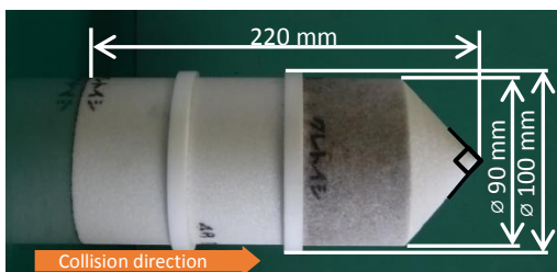
Figure 2 Photo of the conical type abrasive projectile used for the collision experiment (2.8 kg)
